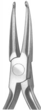
DTICP-2653 How Plier Tips are 1/8" (3.2mm) diameter
